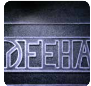
Cold soda lime glass cutting
